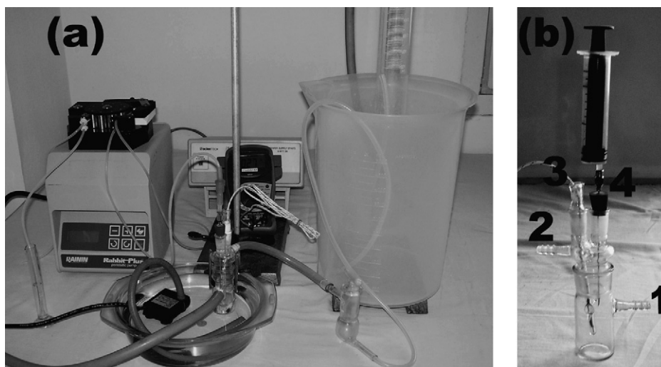
Fig. 1. (a) Experimental set-up. (b) Reactor: (1) argon inlet for flushing; (2) hydrogen outlet; (3) temperature sensor; (4) \text{NaBH}_4 solution inlet.
